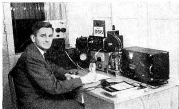
The equipment used by SP5HS includes a BC312 receiver, a home-built double-superhet, a v.f.o. controlled 100 watt transmitter using an RL12P35, a 40m long wire and a 20m dipole for operation on 20m, 40m and 80m c.w. On 2m, the crystal controlled transmitter runs 100 watts input to an 829B. The converter, also crystal controlled, uses an ECC84 and an ECC85. The present aerial is a 4-element Yagi but a 28-element array is almost ready for service.
